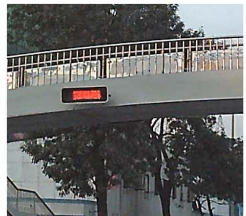
And..in China new LED strips change from green to yellow to red, using one light instead of three. The strip is fully illuminated at the start of each signal, then shrinks in size to show how much time is left before the color changes.
