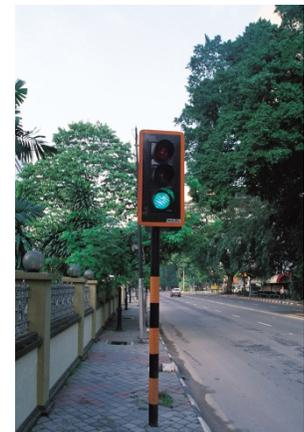
Another area of innovation is related to the light source. Traditionally, incandescent and halogen bulbs were used. But, because of the low efficiency of light output, newer designed incorporate LED arrays that consume less power, have increased light output, last significantly longer, and in the event of an individual LED failure, still operate although with a reduced light output.
